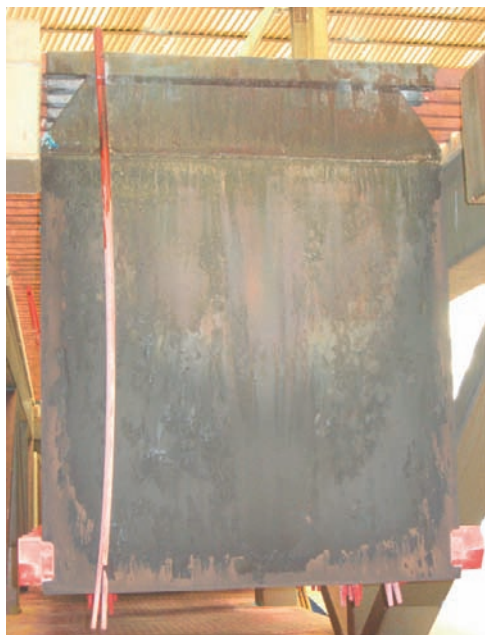
FIGURE 17.3 Pb-alloy anode. Note the insulator strips hanging on each side of the anode and the insulator buttons on the side. These prevent short circuiting between the anode and cathode and assist in placing the anodes vertically and straight in the cells.
