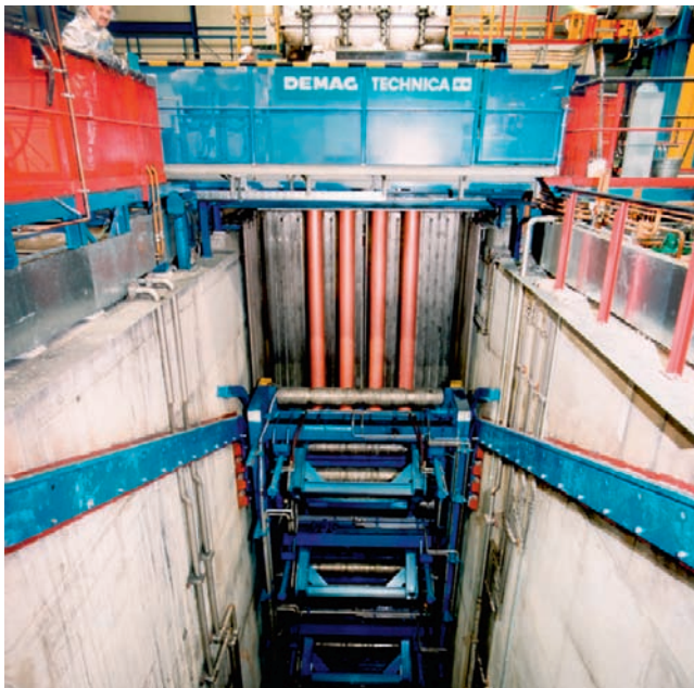
FIGURE 20.3 Semi-continuous vertical chill caster for extrusion. (Courtesy SMS Meer, 2008.)
