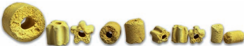
FIGURE 12.5 Photograph of catalyst pieces. The outside diameter of the largest piece (far left) is 20 mm. Pellets are shown far right, rings in the middle, and 'daisy' shapes (modern) left and right of the rings. (Courtesy Haldor Topsoe A/S.)
