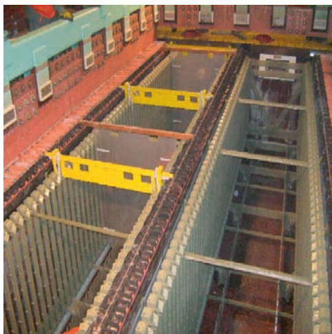
FIGURE 17.7 SELE cathode holder maintains accurate positioning and electrode alignment in EW cells for high current density applications.
