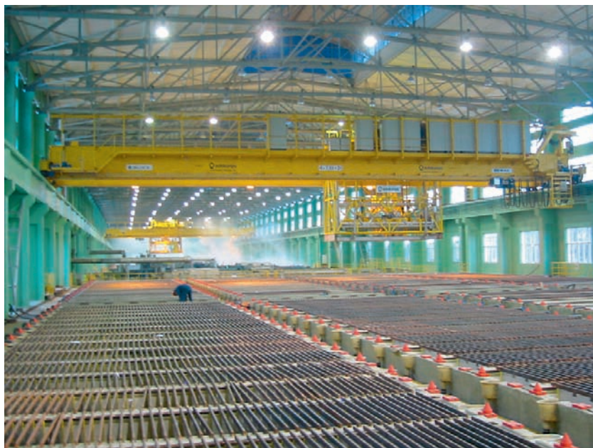
FIGURE 14.2 A modern copper electrorefinery in China. Note the overhead crane used for moving anodes and cathodes to and from the cells. In the background, the plastic sheets covering some of the cells minimize evaporation and heat losses, thereby minimizing energy consumption. (Courtesy of Outotec.)
