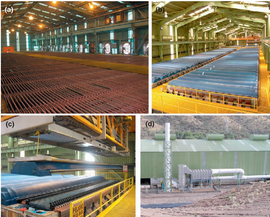
FIGURE 17.8 Tankhouse equipment to avoid and mitigate the effects of acid mist. (a) Older tankhouses use extraction fans and ventilation across the cells, while (b) modern tankhouses use hoods to cover the cells. These are lifted for harvesting of cathodes (c), requiring very accurate positioning, so computer control of the crane movements is essential. (d) The acid mist is captured and scrubbed to avoid releasing corrosive gases to the environment. (Photos (b) and (d) courtesy of Outotec.)
