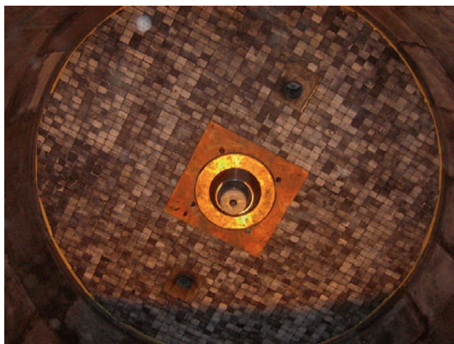
FIGURE 10.1 New Chingola direct-to-copper flash furnace. The photo shows the top of the reaction shaft and the bottom tip of the concentrate burner. The diameter of the reaction shaft is ~6 m. Photograph by W.G. Davenport.
