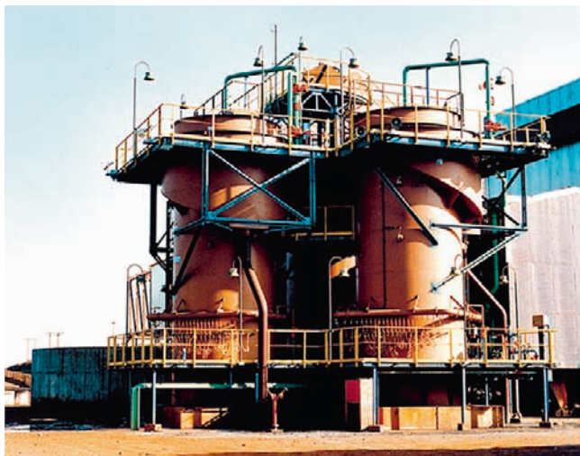
FIGURE 4.7 Industrial column flotation cells. Their sizes around the world are given in Table 4.4.
